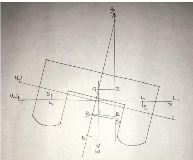
Figure 6: Stability at a large angle
