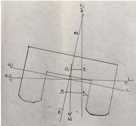
Figure 4. effect of large angle of heel on a catamaran
