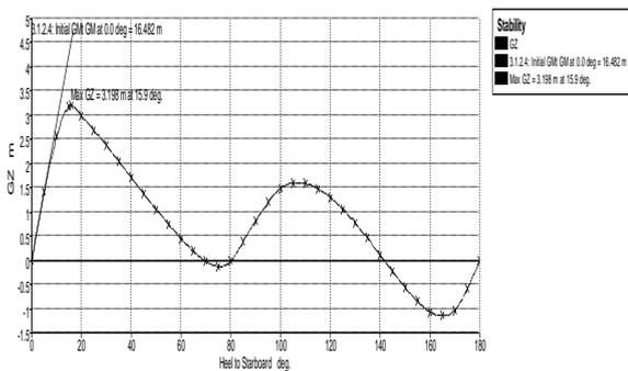
Figure 20: Statical stability curve for loadcase 3
