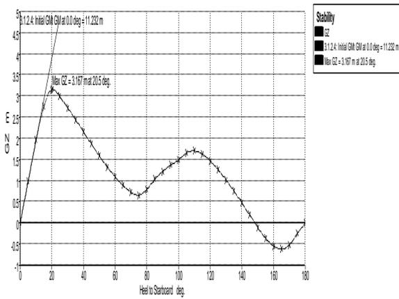
Figure 18: Curve of statical stability for load case 1
