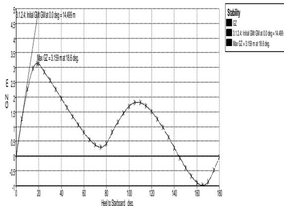
Figure 19: Statical stability curve for load case 2
